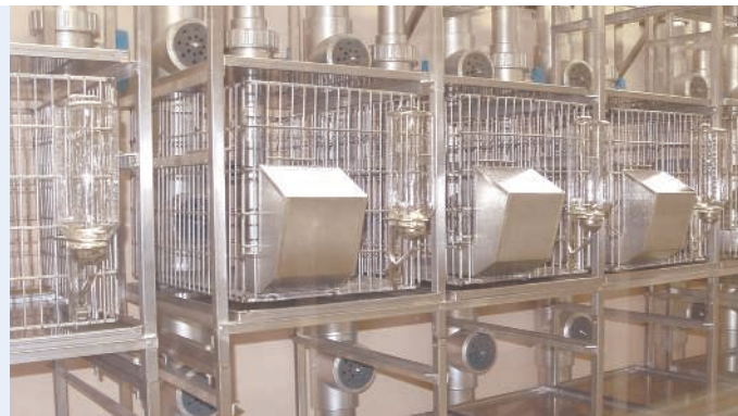
Transmission. Air from a TB ward is vented into guinea-pig cages ( above ) at an experimental facility in Witbank.
